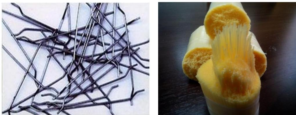
**Figure 2.** (left) Steel fiber and (right) Synthetic (polypropylene) fiber.
