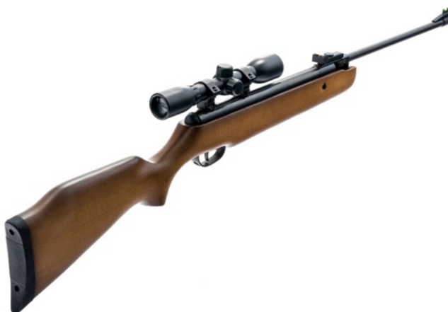
Figure 10. Pellet gun used to introduce impact damage.
