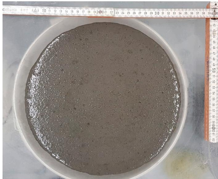
Figure 3. AS/B.18 mix during flow test.
