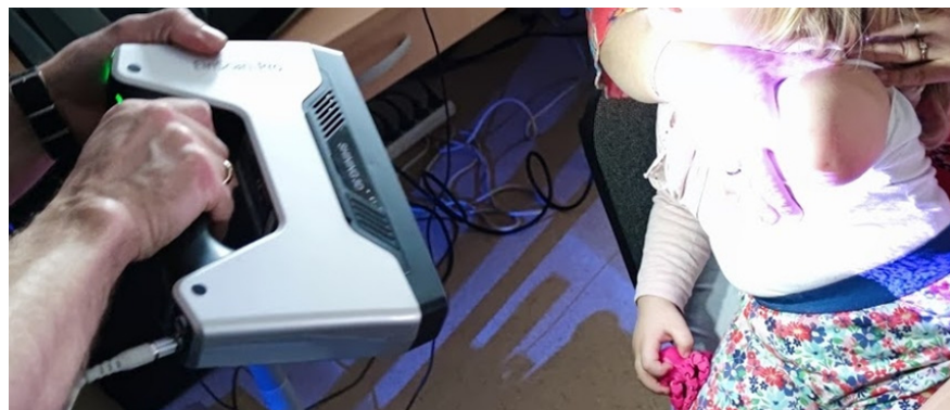
Figure 4. Manual 3D scanning of the patient's stump.
