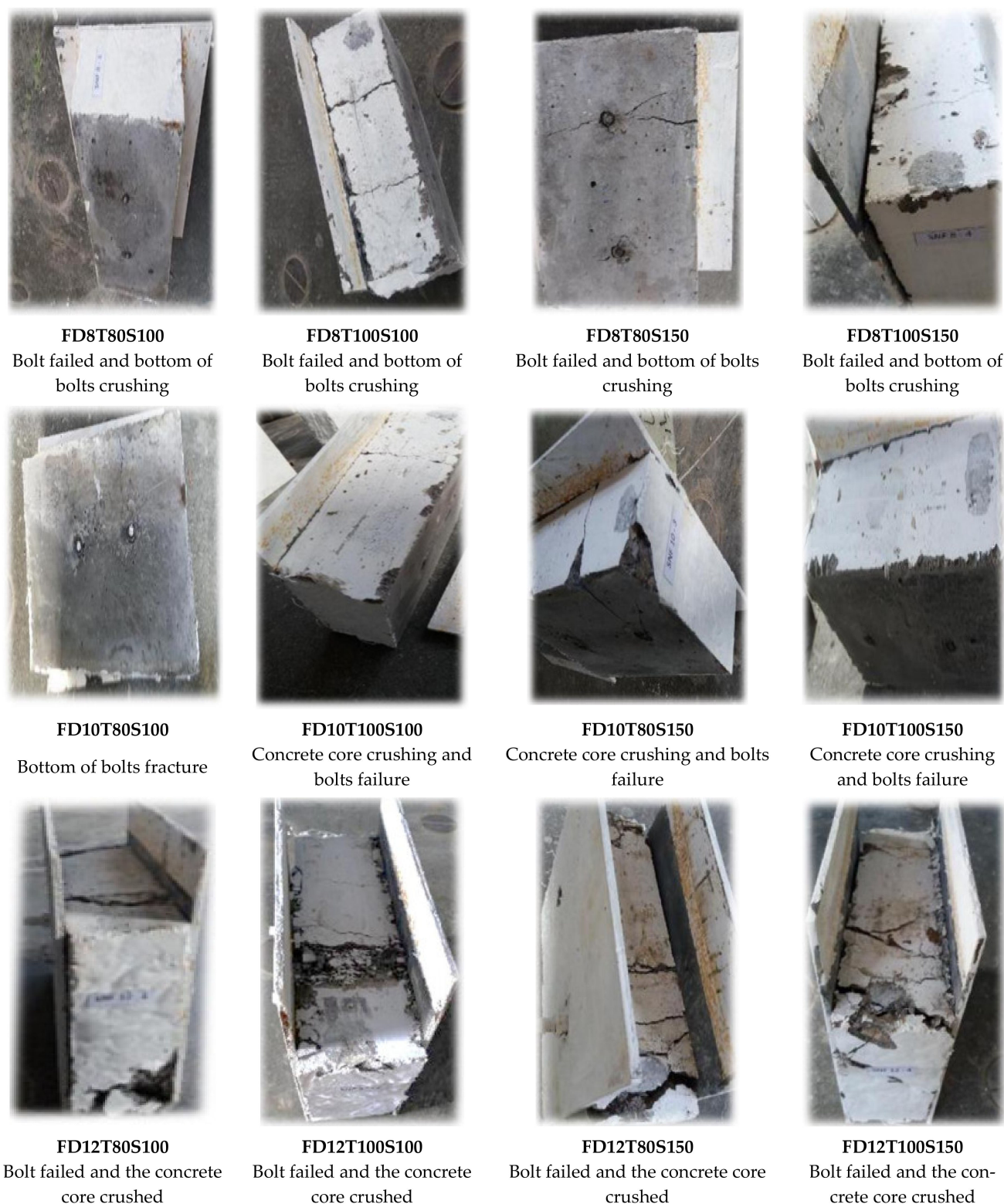
Figure 9. Typical static failure modes of specimens with and without SF.
