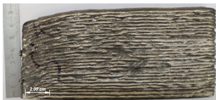
Figure 11. The wall appearance, mode I = 120 A, U = 20 V.
