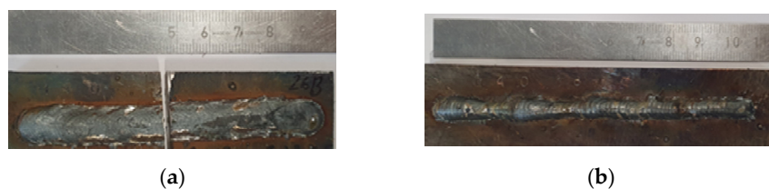
Figure 9. The appearance of the bead, (a)— I = 120 A, U = 26 V; (b)— I = 120 A, U = 18 V.
