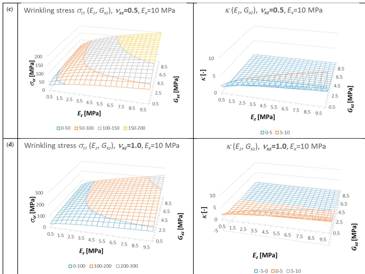
**Figure 8.** Influence of core material parameters on the value of wrinkling stress and the parameter  $\kappa$ : (a)  $\nu_{xz} = -1.0$ , (b)  $\nu_{xz} = 0$ , (c)  $\nu_{xz} = 0.5$ , (d)  $\nu_{xz} = 1.0$ .
