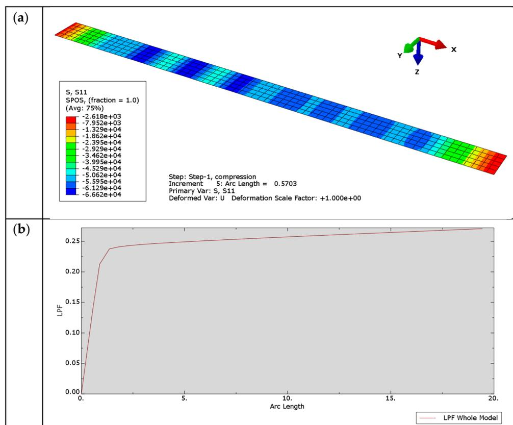
**Figure 6.** Numerical solution of the compression of the elastic facing resting on the susceptible core: (a)  $\sigma_x$  stress at the top of the facing (fifth load increment) (b) LPF–arc length relation.
