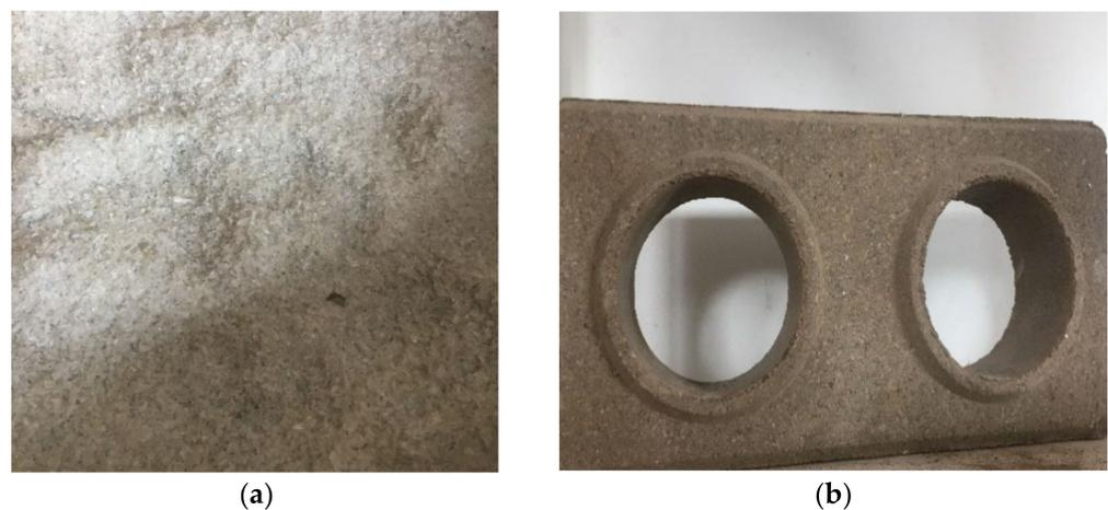
**Figure 1.** Materials used: (a) PET waste; (b) soil-cement brick.
