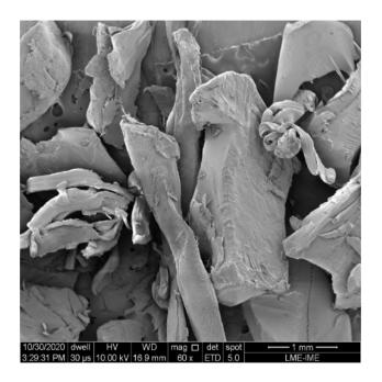
Figure 5. Scanning Electron Microscopy (SEM) of PET 60× magnification.
