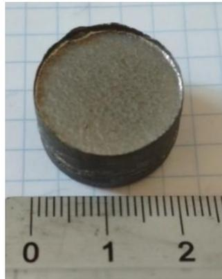
**Figure 2.** Photograph of spark plasma sintered zirconium sample with dimensions  $\text{Ø}20 \times 30$  mm.
