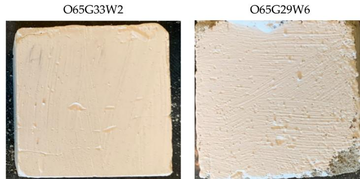
**Figure 10.** Testing the adhesion of adhesive mortar to concrete.
