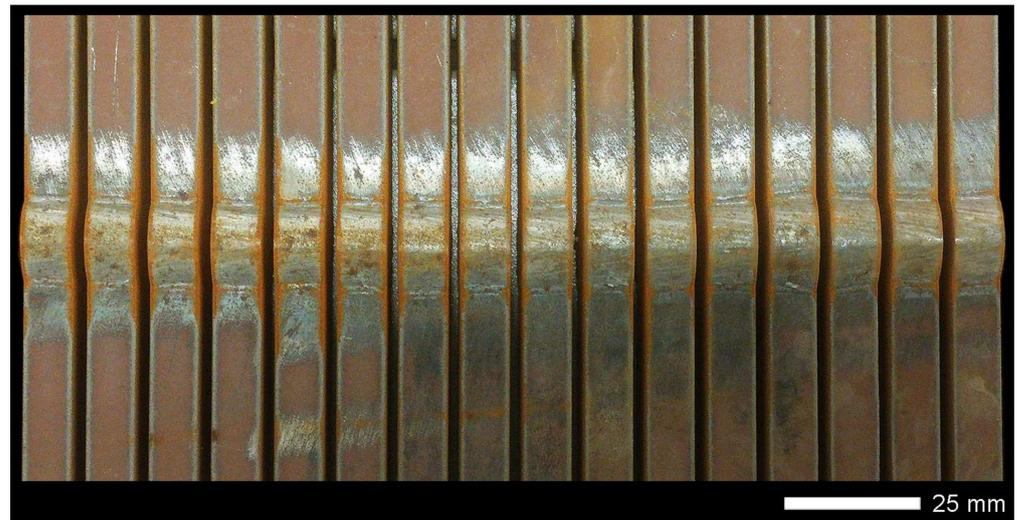
**Figure 6.** A fragment of a welded joint of Hardox 600 steel after the operation of cutting rectangular specimens from the weld area using a high-energy liquid stream with abrasive.
