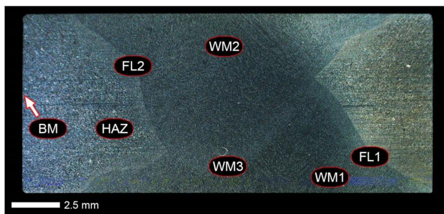
**Figure 29.** Macroscopic image of the welded joint cross-section of Hardox 600 in the heat-treated state according to the diagram No. 9 shown in Table 6. WM—weld metal zone, FL—fusion line, BM—base material zone, HAZ—heat-affected zone. Stereoscopic microscopy, etched with 3% HNO<sub>3</sub> in ethyl alcohol.
