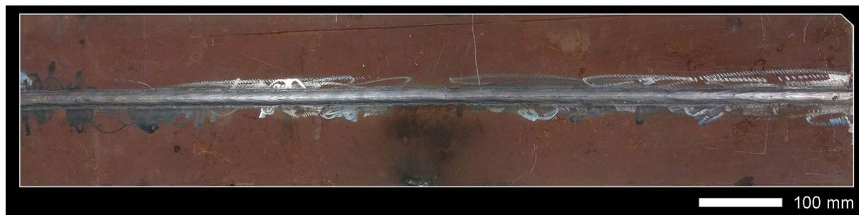
**Figure 4.** A fragment of steel sheets shown in Figure 2 with a welded joint.
