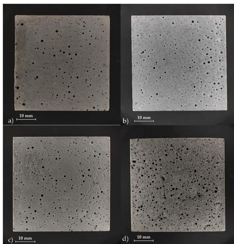
**Figure 3.** Tested concrete samples: (a) REF<sub>SF</sub>; (b) GG<sub>100</sub>; (c) MWG<sub>100</sub>; (d) PG<sub>100/50</sub>.
