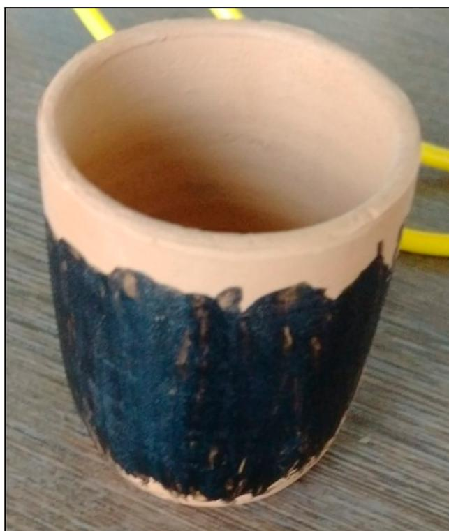
**Figure 3.** Ceramic separator with an electrode coated with graphene air-cathode assembly.
