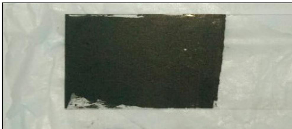
**Figure 1.** Thin-film of castor oil-emitted powder for characterization.
