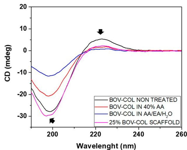
**Figure 3.** Circular dichroism analysis performed on native collagen (BOV-COL NON-TREATED), collagen reconstituted after dissolution in AA/EA/H<sub>2</sub>O (BOV-COL in AA/EA/H<sub>2</sub>O), collagen reconstituted after dissolution in 40% AA (BOV-COL in 40%AA) and collagen scaffolds obtained by processing 25% BOV-COL in 40% AA (25% BOV-COL SCAFFOLD).
