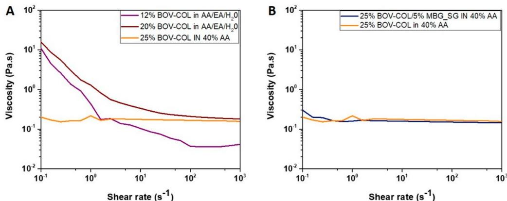
**Figure 2.** Comparison between flow ramps obtained from 12%BOV-COL in AA/EA/dH<sub>2</sub>O, 20%BOV-COL in AA/EA/dH<sub>2</sub>O and 25%BOV-COL in 40% AA (A), and flow ramps of 25%BOV-COL in 40% AA and 25%BOV-COL/5%MBG\_SG in 40% AA (B).
