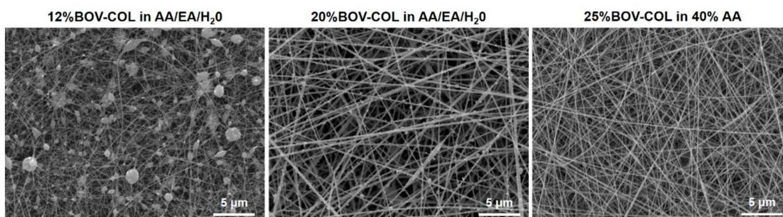
**Figure 1.** SEM images of scaffolds obtained from the electrospinning of 12%BOV-COL in AA/EA/dH<sub>2</sub>O, 20%BOV-COL in AA/EA/dH<sub>2</sub>O and 25%BOV-COL in 40% AA.
