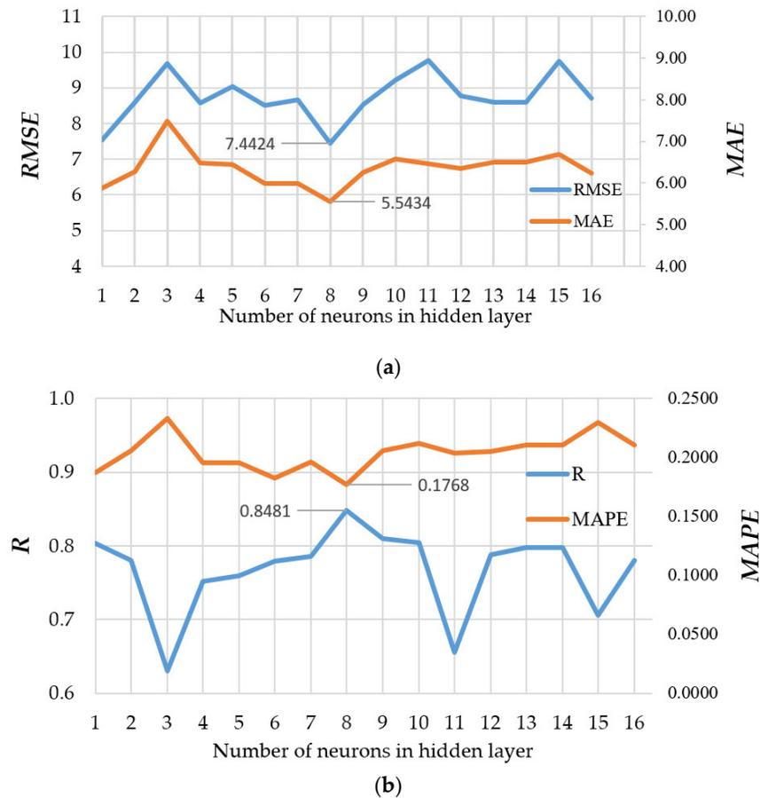
**Figure 7.** Comparison of performance measures using MLP-ANNs with different configurations: (a) *RMSE* and *MAE*, (b) *R* and *MAPE*.
