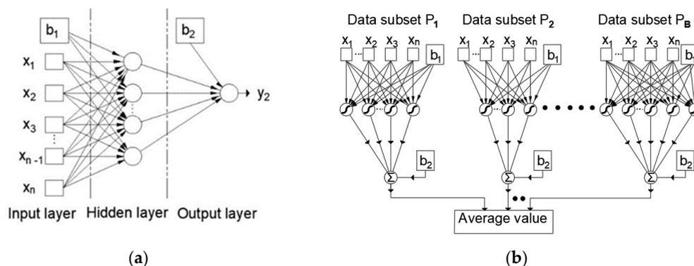
**Figure 1.** (a) Multilayer perceptron artificial neural network; (b) an ensemble of neural networks formed by the Bootstrap Aggregating (Bagging) approach [33,34].
