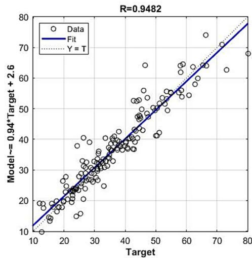
**Figure 19.** Regression plot of modelled and target values of compressive strength for reduced GPR ARD Matern 32 model.
