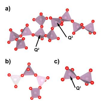
**Figure 12.** Exemplary phosphate network elements for x = 0 (a), x = 25 (b), and x = 50 (c) glasses.
