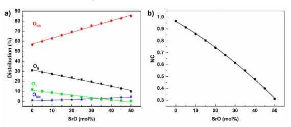
The distribution of the oxygen atom types as a function of the glass composition is shown in Figure 10a.
