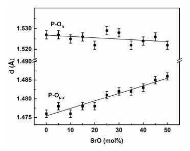
Figure 3. Dependence of P-O<sub>B</sub> and P-O<sub>NB</sub> distances on composition.
