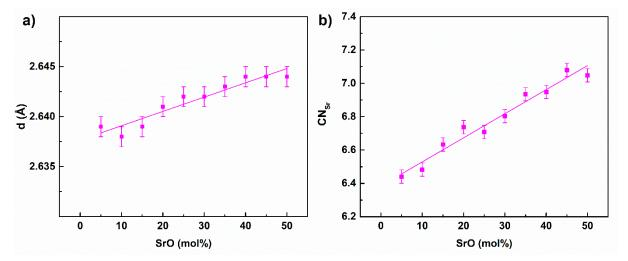
Figure 7. The Sr-O distance (a) and coordination number (b) as a function of the glass composition.
