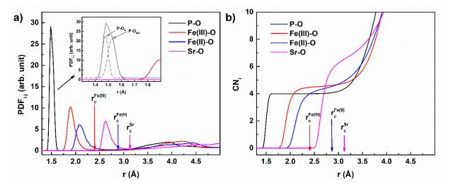
**Figure 2.** The P-O, Fe(III)-O, Fe(II)-O, and Sr-O pair distribution functions (PDFs) for 5 mol% of SrO (**a**) and their corresponding average coordination numbers (CNs) analysis (**b**) as a function of distance.
