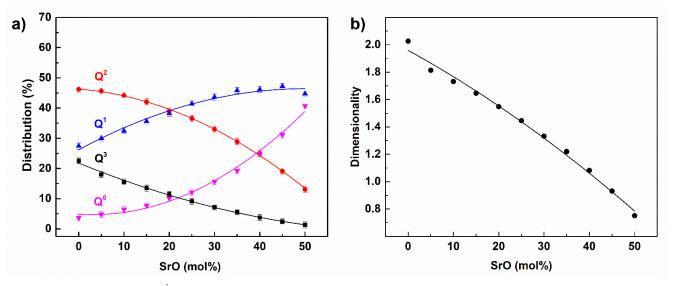
Figure 11. Distribution of Q<sup>i</sup> structural units in the simulated glasses (a) and the dimensionality of the glass network (b).
