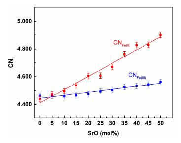
Figure 5. Iron coordination numbers for oxygen vs. SrO content in the glass.
