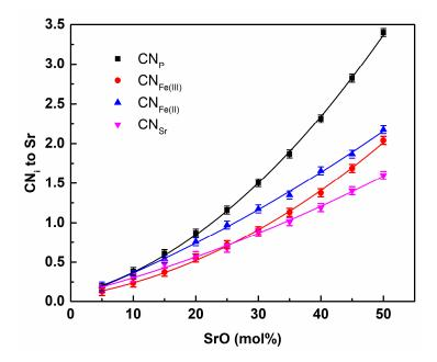
Figure 14. Compositional dependence of the coordination numbers for Ca for P, Fe(II), Fe(III), and Sr.
