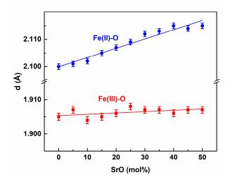
Figure 4. The Fe(III)-O, and Fe(II)-O distances as a function of the glass composition.
