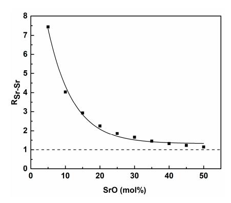
Figure 15. Dependence of the Sr-Sr aggregation parameter (R<sub>sr-sr</sub>) of the glass composition.
