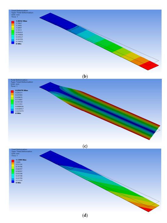
**Figure 9.** FE model of morphing wing with bimorph configuration of MFC actuators. (a) Two MFCs are bonded on the top and bottom surfaces of the cantilever beam. (b) The bending moment resulting from applying different voltages on MFCs. (c) The torsion moment resulting from applying the same voltages on MFCs. (d) The coupled torsional and bending moments resulting from actuating only one MFC from either side.
