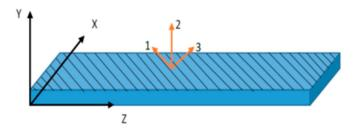
**Figure 4.** Schematic for MFC-F1 type with 45° fiber laminates in the 3-axis and IDE in the 1-axis.
