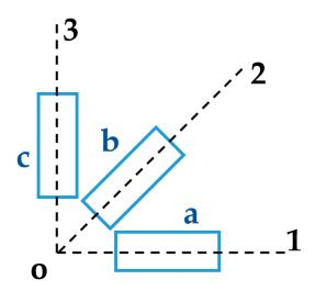
**Figure 10.** Schematic showing three strain gauges (a, b, c) aligned with three axes (1, 2, 3).
