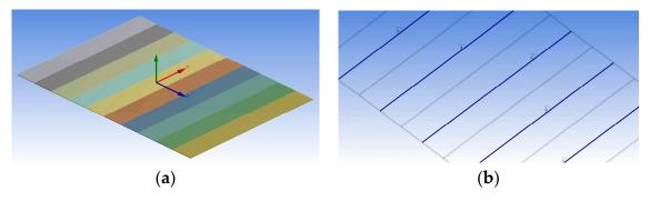
**Figure 3.** (a) FEM of multiple segments of piezoelectric actuators of MFC with the coordinate system. (b) Blue surfaces indicate positive voltage and gray surfaces indicate zero voltage in the finite element model.
