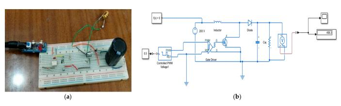
Figure 11. (a) Boost converter circuit; (b) MATLAB-Simscape model for the boost converter.
