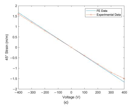
**Figure 15.** Verification of FE simulation strains (m/m) and experimental strains (m/m) due to MFC actuation in volts (V): (a) axial strain ( $\varepsilon_c$ ); (b) transverse strain ( $\varepsilon_a$ ); (c) strain at  $45^\circ$  ( $\varepsilon_b$ ).
