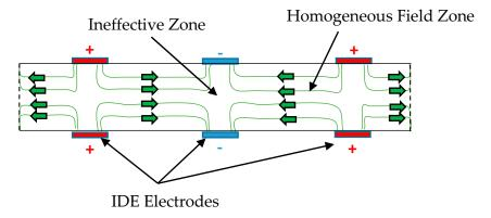
Figure 2. Sketch for the structure of homogenized MFC with interdigitated electrodes.
