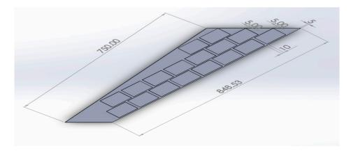
**Figure 16.** CAD model for a sweptback wing with MFC actuators on its surface (dimensions are in mm).
