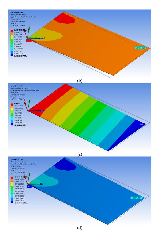
**Figure 8.** Simplified FE model of M-8557-F1 showing (a) the result for elongation displacement in the *z*-axis, (b) the result for max elongation strain, (c) the result for compressive displacement in the *z*-axis, and (d) the result for max compressive strain.
