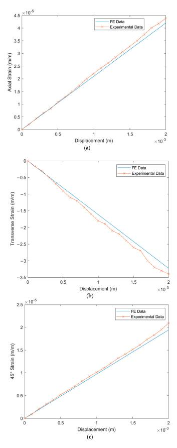
**Figure 14.** Verification of FE simulation strains (m/m) and experimental strains (m/m) due to tip displacements ( $\mu$ m): (a) axial strain ( $\epsilon_c$ ); (b) transverse strain ( $\epsilon_a$ ); (c) strain at  $45^\circ$  ( $\epsilon_b$ ).
