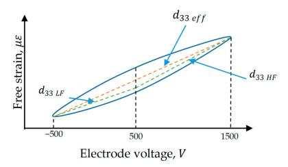
**Figure 1.** Longitudinal free strain versus applied electrode voltage showing the piezoelectric constant variation with the voltage range.
