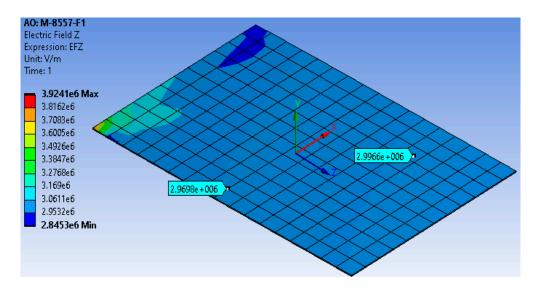
**Figure 7.** Simplified FE model of the electric field generated from the applied voltage difference of 255,000 V, which is equivalent to 1500 V in the physical MFC.
