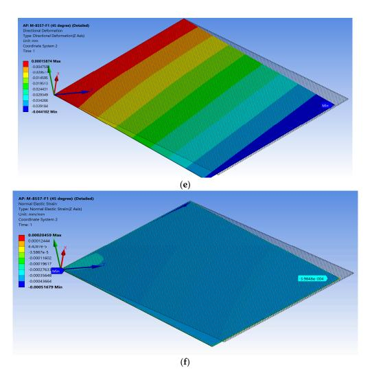
**Figure 6.** Detailed FE model of M-8557-F1 showing (a) applied voltage difference of 1500 V for every segment, (b) the generated electric field of about  $\pm 3 \times 10^6$  V/m, (c) the result for elongation displacement in the *z*-axis, (d) the result for max elongation strain, (e) the result for compressive displacement in the *z*-axis, and (f) the result for max compressive strain.
