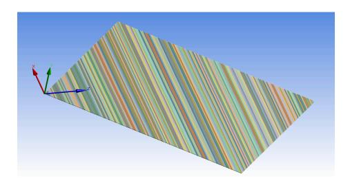
**Figure 5.** Detailed FE model for MFC-F1 type with  $45^{\circ}$  fibers orientation.
