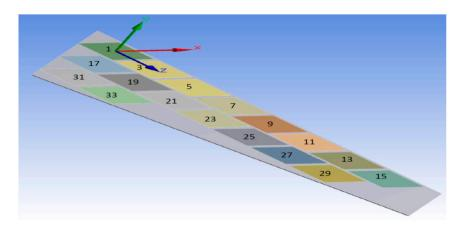
**Figure 17.** FE model of sweptback wing showing numbered MFC actuators and their coordinate system.
