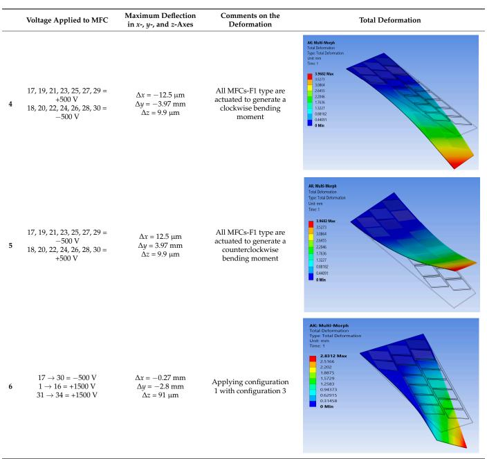
The results show that the proposed FE techniques can analyze efficiently (very low computational time and small memory usage) a variety of morphing wing shapes that are generated with a large number of MFC actuators. This variety of morphing wing shapes can greatly affect lift, pitch moment, and rolling moment, which increases the maneuverability of the associated air vehicle.
