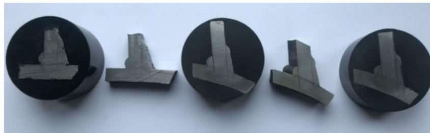
**Figure 12.** Actual weld profile cut from one of the specimens.
