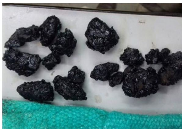
Figure 2. Detachment of the RCA asphaltic mixture.
