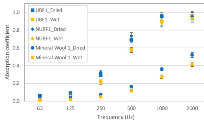
**Figure 5.** Variation in absorption coefficient with the degree of humidity in the analyzed samples (octave bands).
