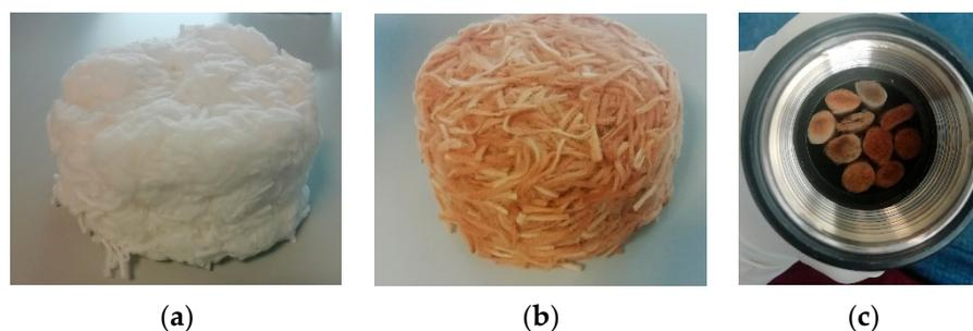
**Figure 1.** Example pictures of some of the prepared samples: (a) sample from disaggregated non-used cigarette butts; (b) sample from disaggregated used cigarette butts; (c) sample from used cigarette butts before the cleaning treatment.
