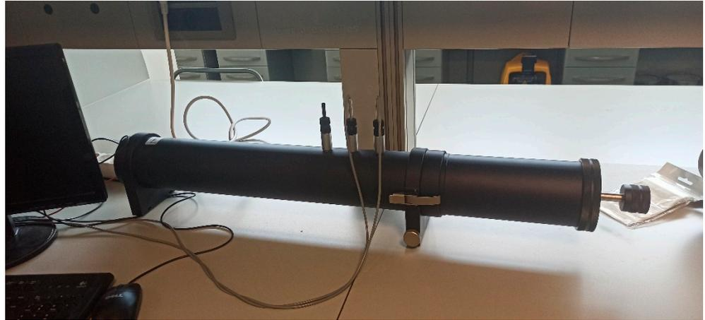
Figure 2. Impedance tube disposition used for the measurements.
