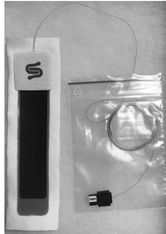
Figure 7. StretchSense™ StretchFABRIC sensor has a fabric substrate. The polymer housing that protects the sensor is affixed to the substrate via an adhesive.
