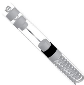
Figure 2. Simplified cross-section of an implantable cardioverter-defibrillator lead.
