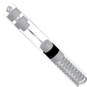
**Figure 2.** Simplified cross-section of an implantable cardioverter-defibrillator lead.
