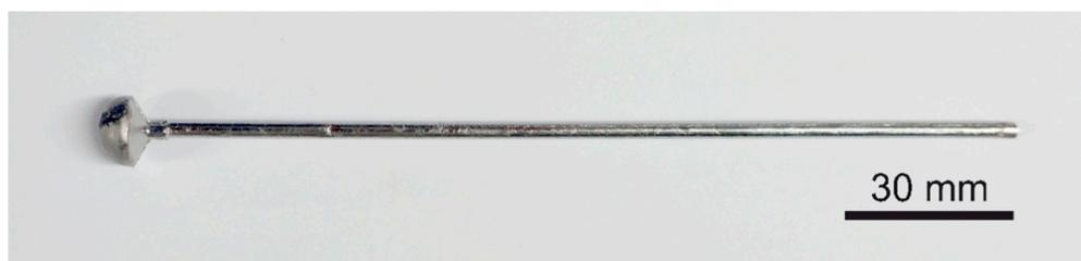
**Figure 2.** The rod obtained by the method of suction casting.
