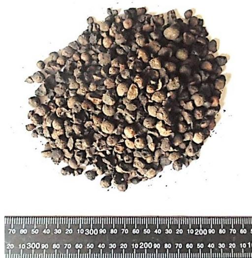
Figure 2. Artificial aggregate Certyd—differentiation of fraction and shape (ruler in mm).
