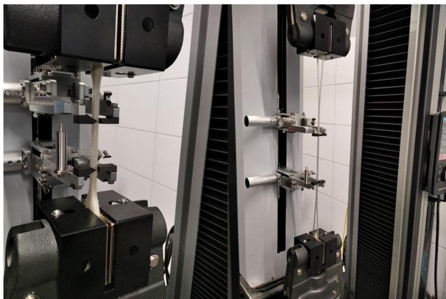
**Figure 11.** Printed sample before and during the static tensile test.
