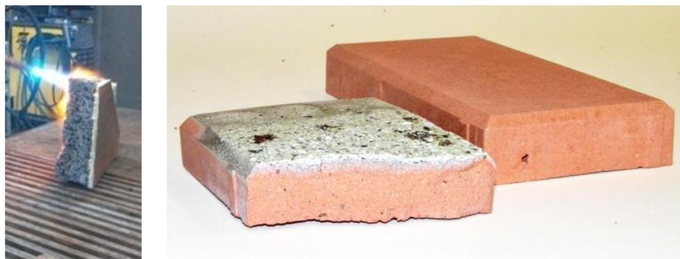
**Figure 5.** Geopolymer materials tested by oxy-acetylene torch (temperature > 3000 °C) (source—own research).
