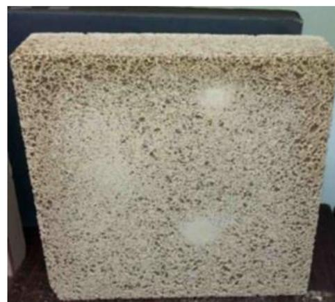
**Figure 3.** Maximum application temperature of some insulation materials, adapted from [12] and an example of foamed geopolymer panel (50 cm × 50 cm) (own research).
