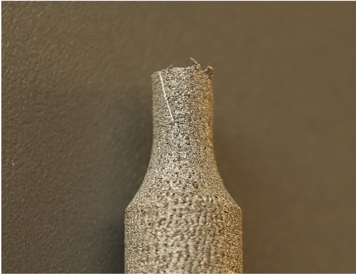
Figure 2. Specimen after the torsional test. Marked line, parallel to the specimen axis before test is inclined to specimen axis. Angle between axis and marked line is shear angle.
