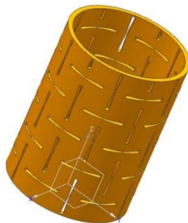
**Figure 6.** Three-dimensional NPR spacer structure.
