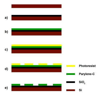
**Figure 1.** Fabrication flow of a parylene-C pattern: (a) growth of a 200 nm  $SiO_2$  layer via thermal oxidation; (b) deposition of a 10–20 nm parylene-C layer; (c) spin coating of a positive photoresist, followed by a 60 s soft bake at 90 °C; (d) development of exposed photo-resist after a 60 s post-exposure bake at 110 °C; (e) etching of unprotected parylene-C in Plasma-Therm and rinsing the residual photoresist.
