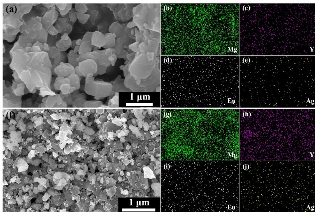
Figure 5. (a) SEM image and (b–e) EDS mapping of  ${}^a\text{MgB}_2 + 0.5\%$   $\text{Y}_2\text{O}_3:\text{Eu}^{3+}/\text{Ag}$ . (f) SEM image and (g–j) EDS mapping of  ${}^c\text{MgB}_2 + 1.2\%$   $\text{Y}_2\text{O}_3:\text{Eu}^{3+}/\text{Ag}$ .
