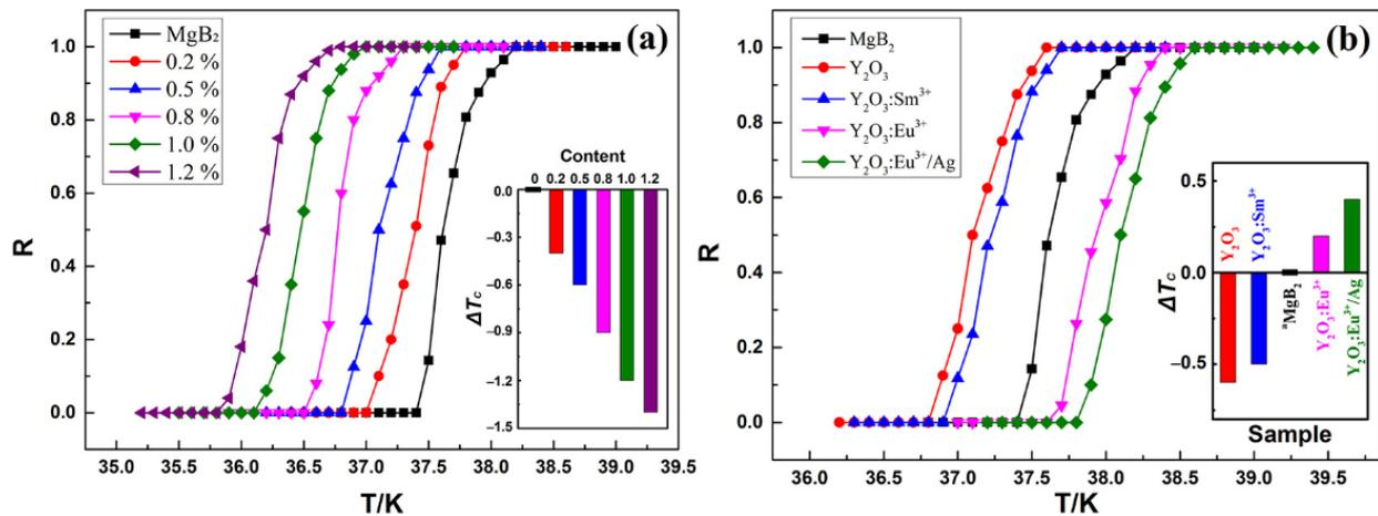
**Figure 3.** Normalized resistivity-temperature curves of <sup>a</sup>MgB<sub>2</sub> doped with (a)  $x\%$  Y<sub>2</sub>O<sub>3</sub> ( $x = 0, 0.2, 0.5, 0.8, 1.0, 1.2$ ) and (b)  $0.5\%$   $y$  ( $y = 0, Y_2O_3, Y_2O_3:Sm^{3+}, Y_2O_3:Eu^{3+}, Y_2O_3:Eu^{3+}/Ag$ ). Insets: the values of  $\Delta T_c$  ( $\Delta T_c = T_c - T_{c\text{pure}}$ ).
