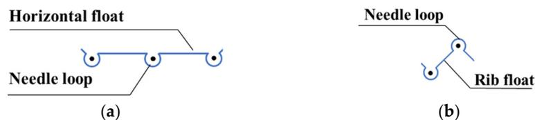
**Figure 3.** Graphical notation of the needle loop, (a) horizontal float and (b) rib float.
