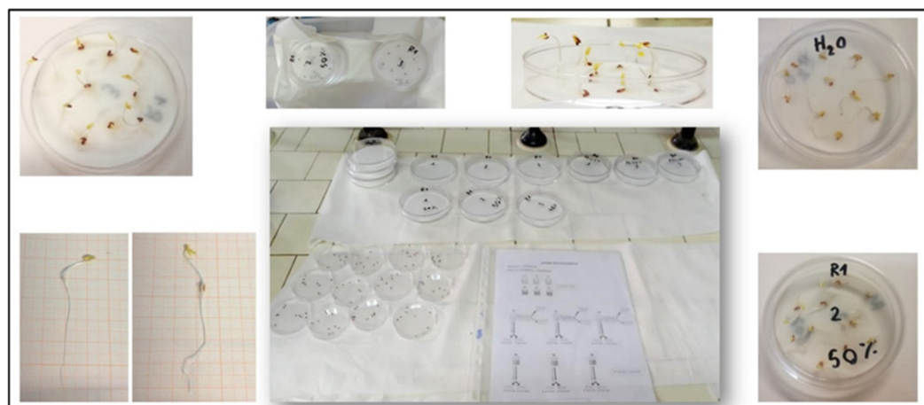
Figure 2. Set-up of the L. sativum seed germination test and germinated seeds after 72 h.
