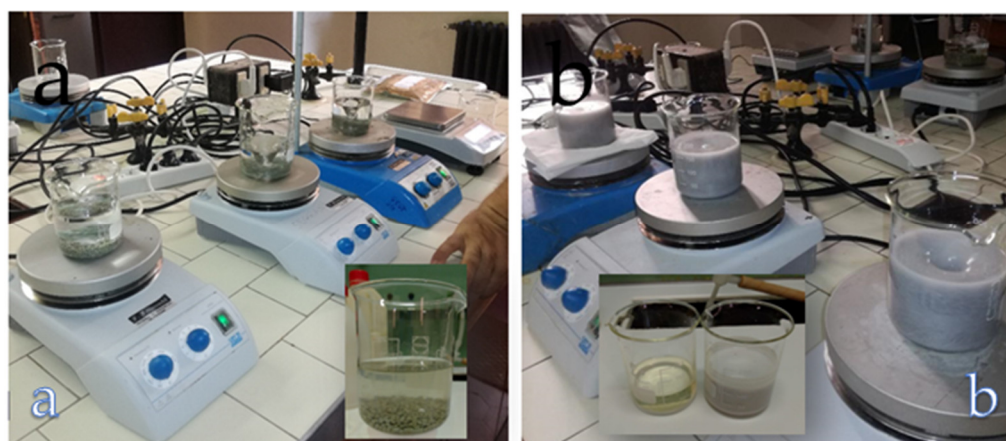
Figure 9. (a) Set-up for the preparation of the eluates and (b) the eluates obtained from PS and graules containing 30 wt.% PS (Matrix1_30).
