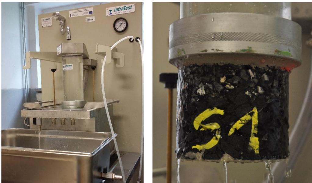
**Figure 6.** Vertical water permeability test.
