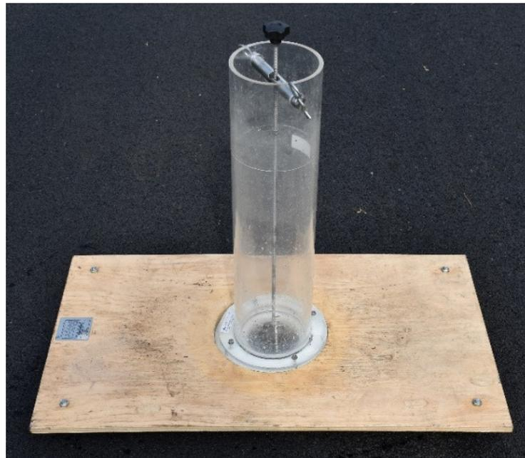
**Figure 5.** Water drainability testing device for the in situ method.
