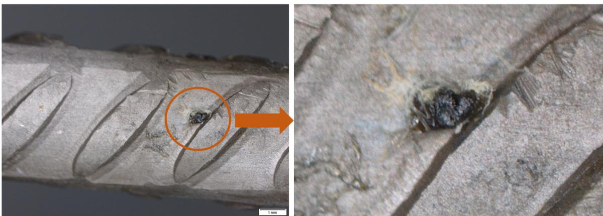
Figure 12. Detail of corrosion in the bar of specimen E11: overview (left) and close-up of a pit (right).
