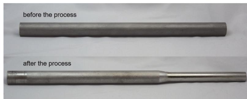
Figure 6. Workpiece before and after rotary swaging.
