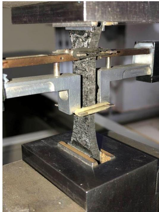
Figure 5. Photograph of tensile specimen and clip-on extensometer.
