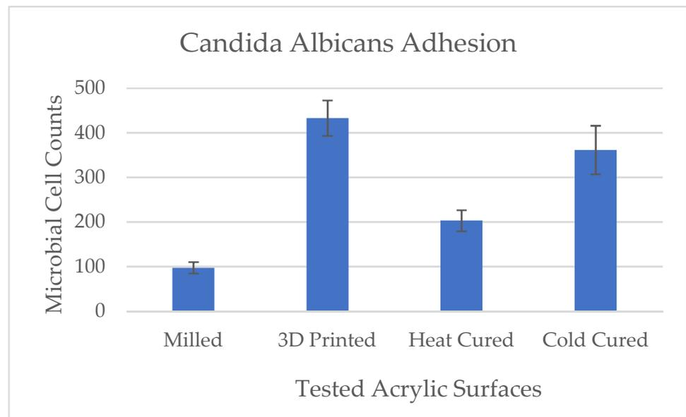
**Figure 5.** Effect of denture acrylic base fabrication method on *Candida albicans* adhesion. Mean results ( $\pm$ standard deviation) are presented as microbial cell counts using morphometric analysis software (ImageJ).
