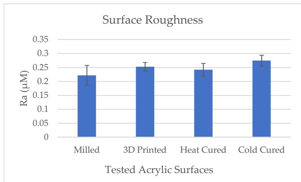
**Figure 2.** Effect of denture acrylic base fabrication method on surface roughness. Mean results ( $\pm$ standard deviation) are presented as Ra ( $\mu\text{M}$ ) measured using profilometric software ( AliconaTM).
