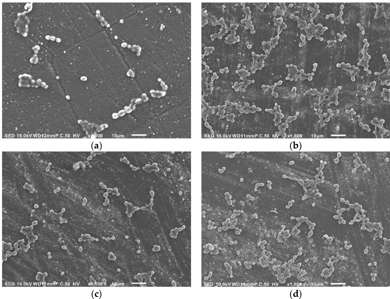
**Figure 6.** SEM images ( $\times 1000$ ; JSM-IT100, Jeol) following microbial adhesion assay for the denture base acrylic samples fabricated using: (a) computerized milling, (b) 3D printing, (c) heat curing, and (d) cold curing.
