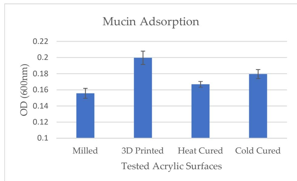
**Figure 4.** Effect of denture acrylic base fabrication method on mucin adsorption. Mean results ( $\pm$ Scheme 600 nm).
