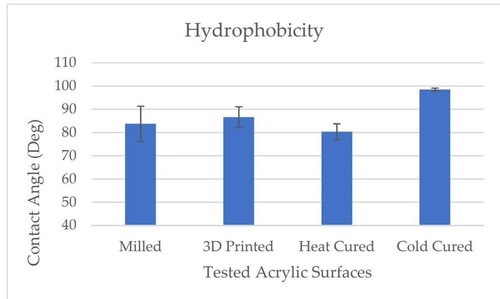
**Figure 3.** Effect of denture acrylic base fabrication method on surface hydrophobicity. Mean results ( $\pm$ standard deviation) are presented as the contact angle measured using a goniometer (Ramé-Hart).
