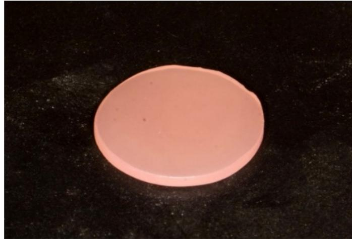
**Figure 1.** Image of milled denture base acrylic discs (CAD\CAM, Vira Vionic Base, VITA).
