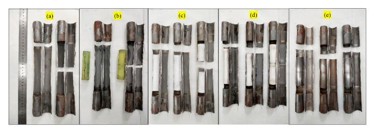
Figure 11. Longitudinal section of the fractured specimen. (a) Longitudinal cross-sectional view of empty tube test specimen. (b–e) The longitudinal cross-sectional views of the specimens when the tube fillers are PU, PTFE, ABS and Q235 respectively.
