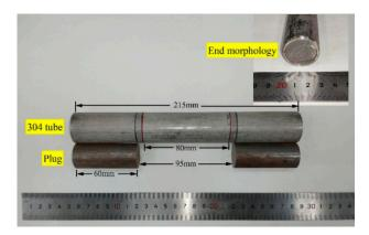
Figure 1. Standard specimen of a 304 SSTWT.
