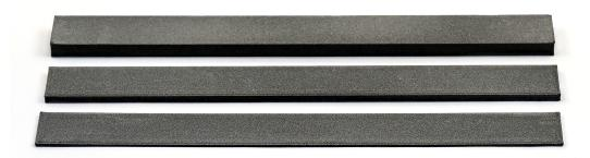
Figure 3. Overview of investigated specimen of three different thicknesses (6 mm, 3 mm, 1 mm).
