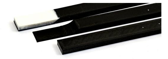
**Figure 2.** Overview of beam specimens with different system complexity: simple beam structure made of PLA (front), beam structure with an ABH made of PLA (center), and beam structure with an ABH made of PLA with an additional damping treatment made of an thermoplastic polyurethane (**back**).
