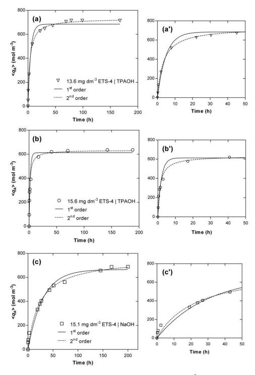
**Figure 4.** Experimental (symbols) and modelling (lines) results of Hg<sup>2+</sup> concentration in the solid phase *versus* time. Experimental conditions: (**a**) TPAOH solution, 15.6 g m<sup>-3</sup> of ETS-4 (O); (**b**) TPAOH solution, 13.6 g m<sup>-3</sup> of ETS-4 ( $\bigtriangledown$ ); (**c**) NaOH solution, 15.1 g m<sup>-3</sup> of ETS-4 ( $\square$ ). On the right side (**a'-c'**), the zoom-in for the first 50 h of each system is shown.
