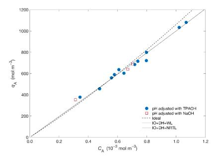
**Figure 1.** Equilibrium data (symbols) and isotherm modelling (lines) results for the system  $Hg^{2+}/Na^+/ETS-4$ . Acronyms: IO = Ioannidis et al. approach, DH = Debye–Hückel, WL = Wilson.
