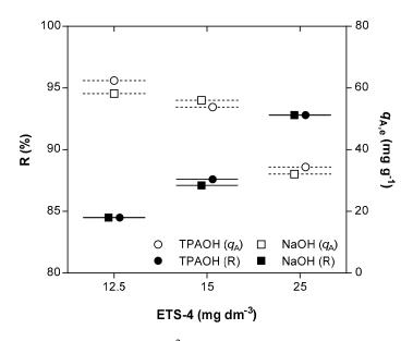
**Figure 3.** Removal (R) of Hg<sup>2+</sup> (black symbols) and equilibrium concentrations of Hg<sup>2+</sup> in the solid phase  $(q_{A,e})$  (white symbols) as function of ETS-4 dose, when using TPAOH (circle) or NaOH (square) as pH adjusting solution. All data refers to the final equilibrium conditions attained.
