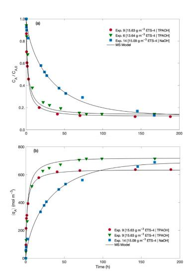
**Figure 2.** Experimental (symbols) and MS model (lines) results along time for (**a**) normalized  $Hg^{2+}$  concentration in the fluid, and (**b**) in the solid.
