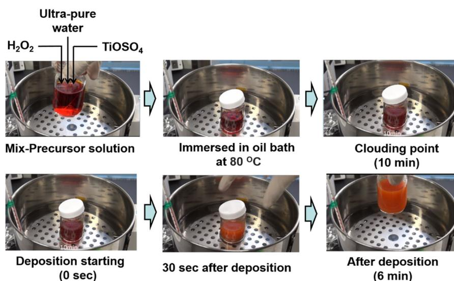
**Figure 2.** Photographs illustrating the hydrolysis steps in chemical bath deposition of TiO<sub>x</sub> films.
