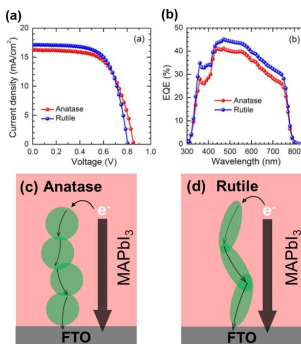
**Figure 6.** (a)  $J$ - $V$  curves and (b) incident photon-to-current efficiency (IPCE) spectra of devices containing anatase and rutile TiO<sub>2</sub> thin films. Schematic of electronic behavior of devices with (c) anatase TiO<sub>2</sub> and (d) rutile TiO<sub>2</sub> films. Reproduced with permission [88]. Copyright 2014, Royal Society of Chemistry.
