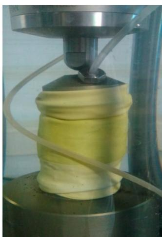
**Figure A7.** Sample of molding sand after tests in triaxial compression apparatus.
