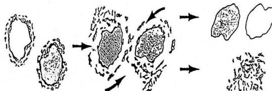
Figure A3. Schematic diagram of matrix release from coatings of used binding material—result of elementary rubbing operation [3].
