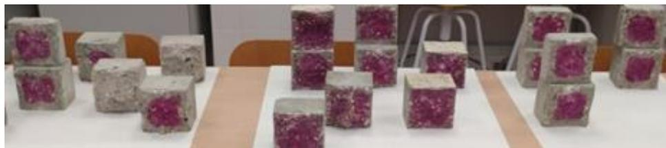
Figure 11. Carbonated SCC probes.
