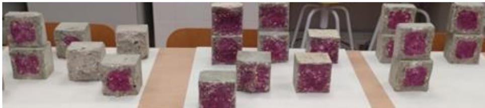
Figure 11. Carbonated SCC probes.
