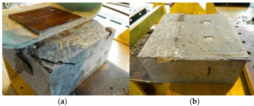
**Figure 12.** Failure mode of specimen S3: (a) concrete surface protrusion crushed; (b) concrete surface—no cracks.
