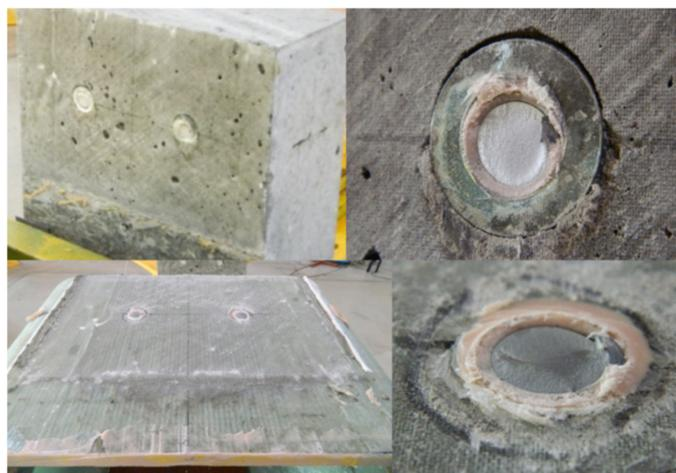
**Figure 9.** Failure mode of specimen S1: concrete surface—no cracks (**top**); GFRP surface—no bearing or shear-out failure (**bottom**).
