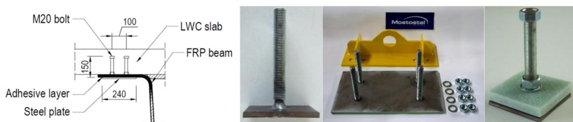
**Figure 2.** Idea and elements of novel shear connection system.
