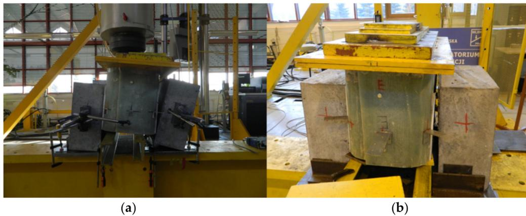
**Figure 7.** Failure modes: (a) static failure of specimen S1; (b) fatigue failure of specimen F4.
