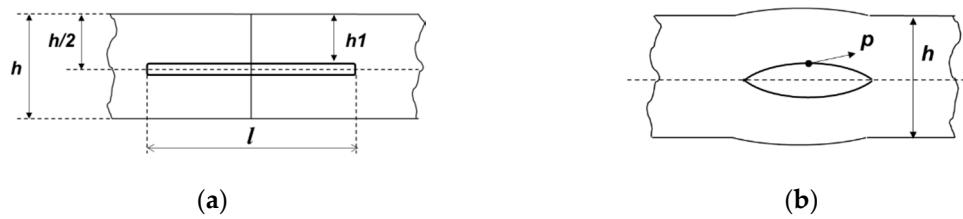
Figure 1. Scheme of the formation of a cavity: (a) Initial position of the notch before being subjected to an internal pressure load p ; (b) Opening of the notch under pressure.
