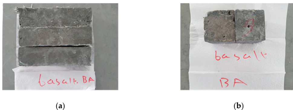
Figure 2. Basalt-fiber-enriched bottom ash composites: (a) flexural samples; (b) cubic samples.
