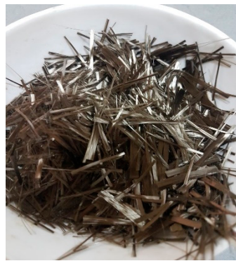
Figure 1. Basalt fiber used in this study.
