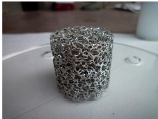
Figure 2. Cylindrical foam sample ( d = 35 mm; h = 35 mm).
