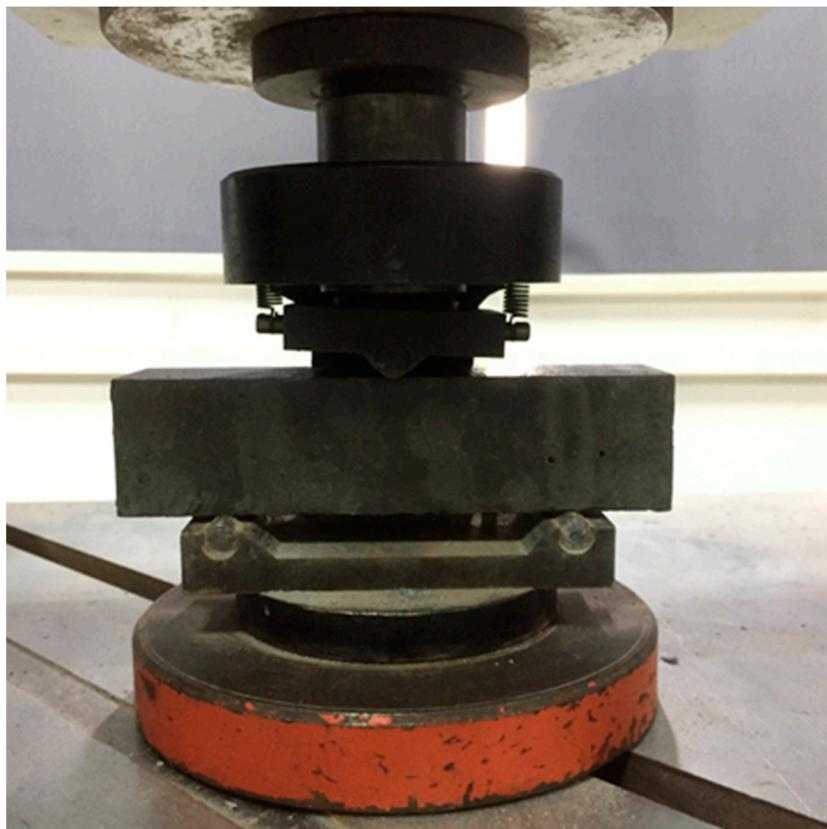
**Figure 3.** Test set-up for flexural strength test.
