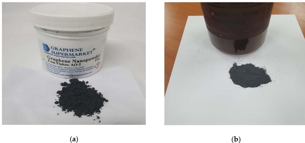
Figure 2. Photograph of nano powder: (a) graphene and (b)  $\text{Al}_2\text{O}_3$ .
