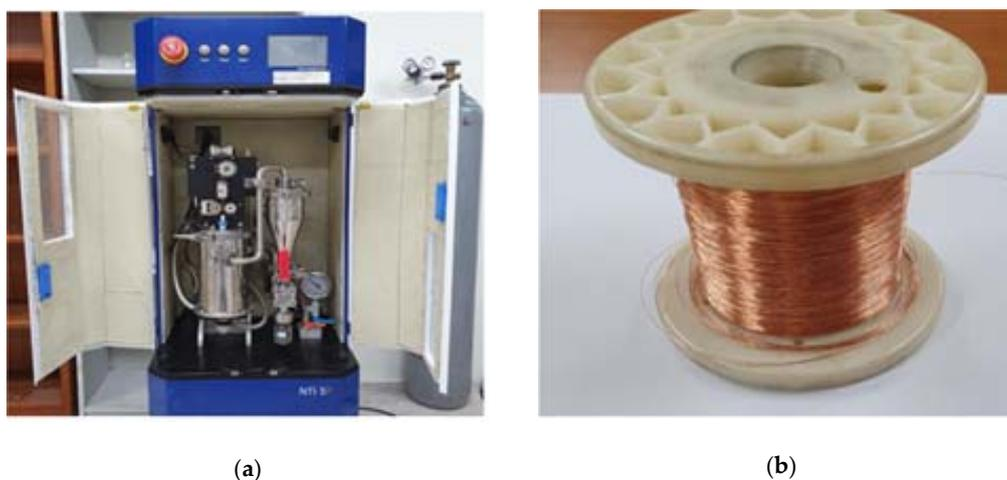
**Figure 1.** Pulsed wire evaporation (PWE) equipment used to manufacture nano powder: (a) photograph of PWE equipment and (b) photograph of copper metal wire used in PWE equipment.
